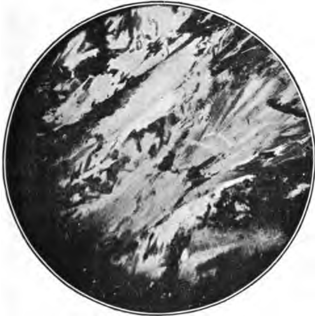
Photomicrograph of Serpentine (Section 42) Showing the divergent arrangement of fibrous structure of the serpentine.
